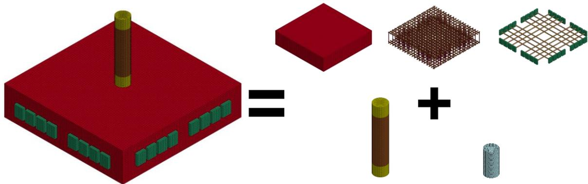
Fig. 1 Finite element model for un-deformable and deformable missile impact
